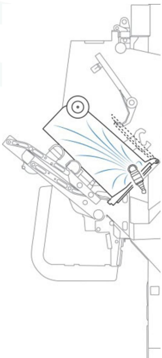
The **MUT ABRA** is our solution for the integrated cleaning of two-wheel and four-wheel containers during your tour. The system can be installed both in press plate vehicles (PRESS MUT, MEGA MUT and Cleanbody) and in rotary drum bodies. The water tanks are positioned between the cab and the body.
